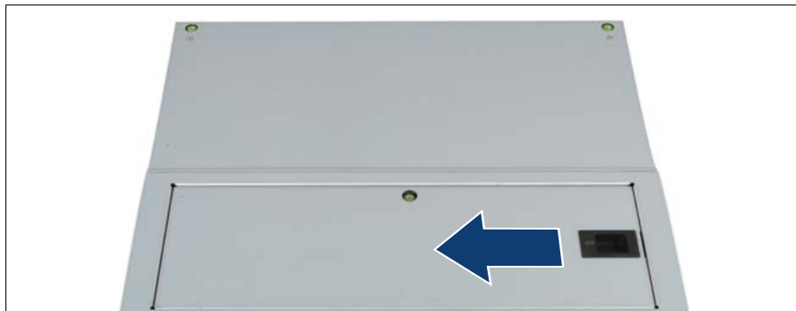
Figure 51: Closing the fan cover
